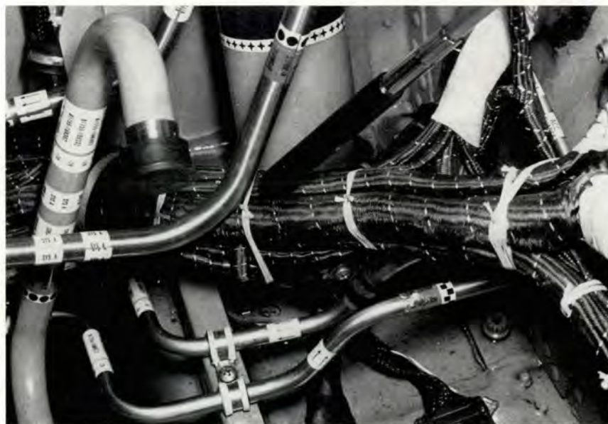
In contrast to hydraulic system leaks, any maintenance or safety person can tell you wire chafing problems are common. As shown above, wire bundles against structure remove insulation and erode metal. If undetected, the potential for an electrical fire exists. Our safety data base reveals we have had 225 chafing-related mishaps in the last 10 years.
